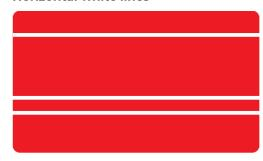
· The ribbon is not correctly fitted.
